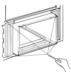
Attach the window locking bracket with a 5/8" screw.
